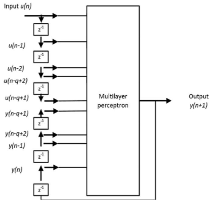
**Figure 4: Non Linear Auto Regressive Model with Exogenous Inputs**
