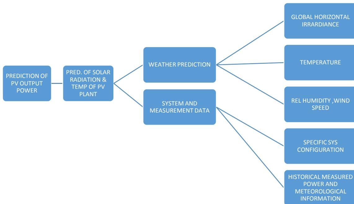
**Figure 1: Typical Framework of various approaches in this type of PV Forecasting.**
