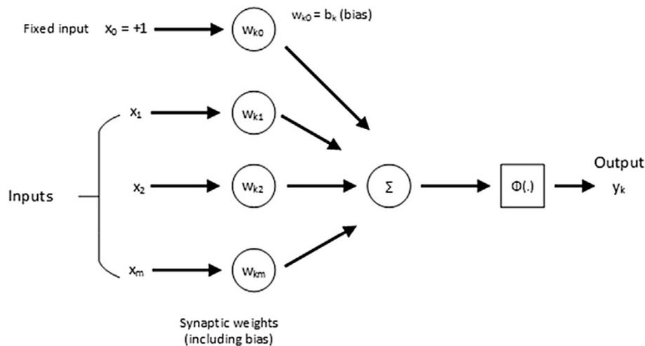
**Figure 3 : Nonlinear model of a neuron (Source:Hayline,1999).**
