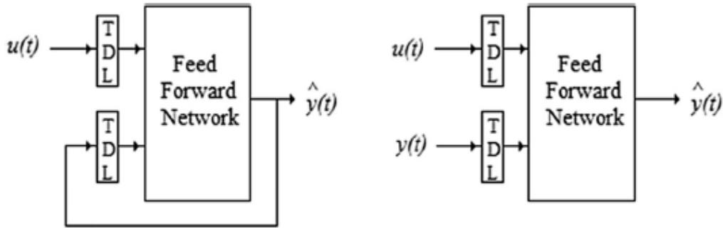
Figure 5: a) Series Parallel Architecture      b) Parallel Architecture
