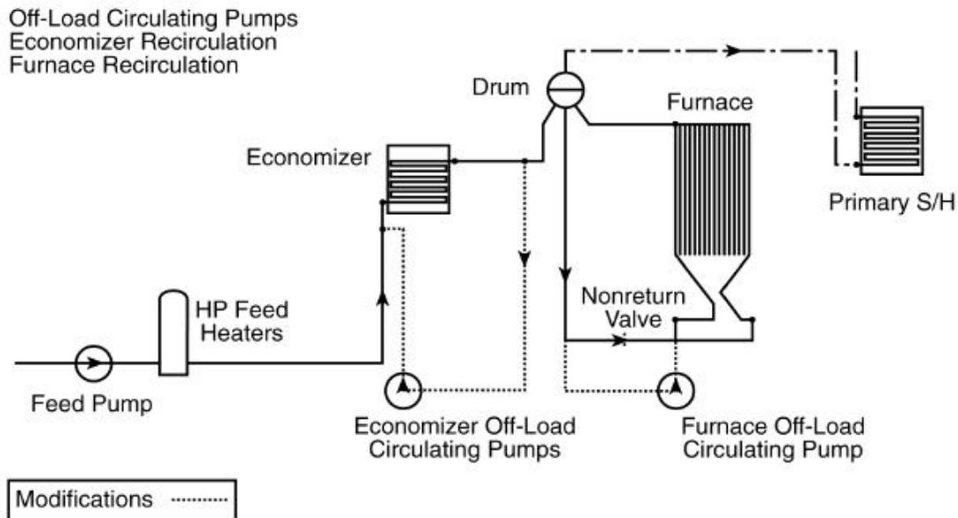
Figure 4: Economizer off-load recirculation pump and furnace off-load recirculation pump.
