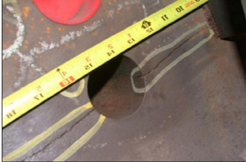
**Figure 3: Cracking in economizer header attributed to severe thermal gradients**
