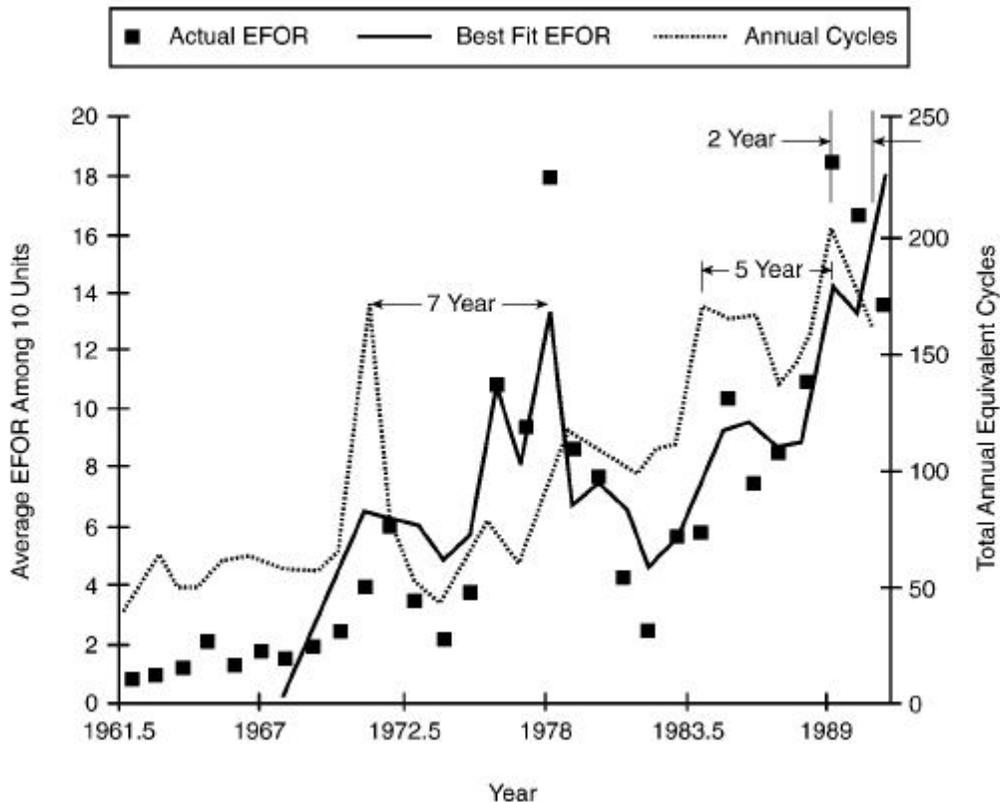
Figure 1: Relationship between cycling and EFOR (Courtesy: Aptech, United States)
