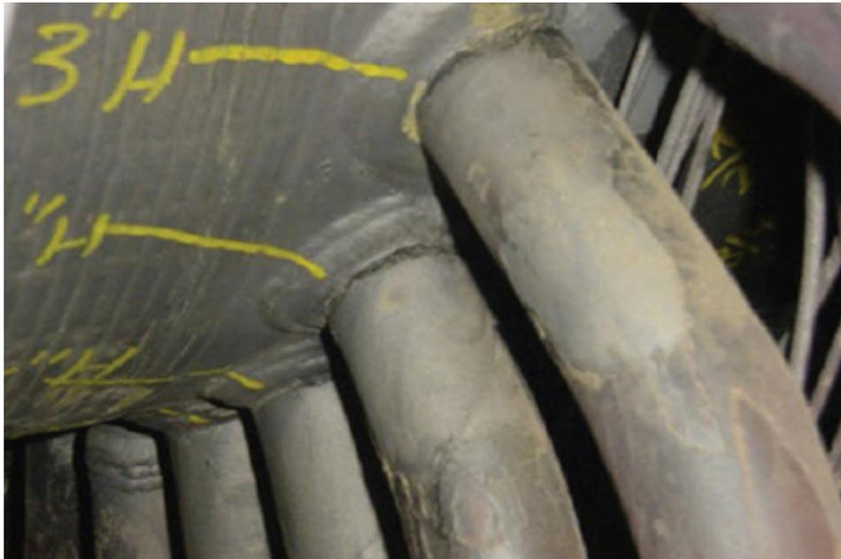
**Figure 2: Water wall damage attributed to severe thermal gradients**
