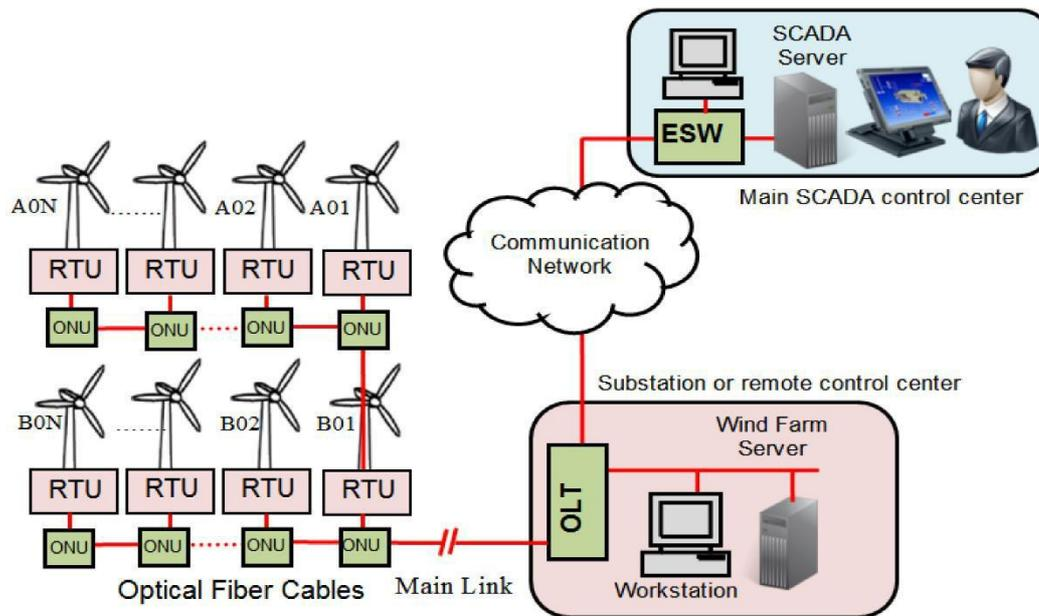
**Fig.1:** Connection of wind turbines in a network
