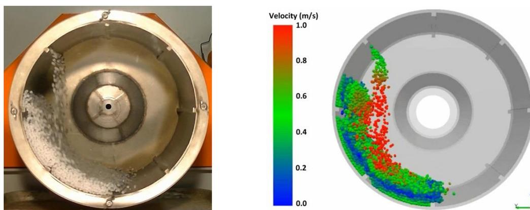
**Figure 4:** AS4156.6 (2000) Dustiness Test: Experiment (left); DE Simulation (right)
