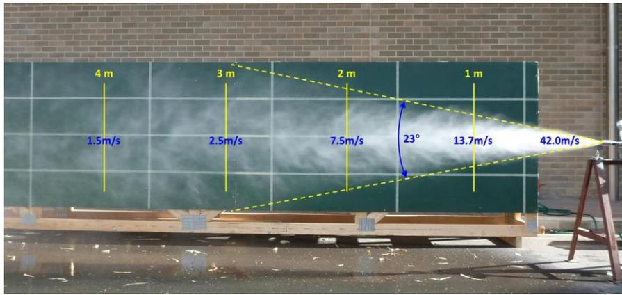
**Figure 5:** Characterisation and Modelling of new EnviroMist High-Energy Micro-Mist Nozzle
