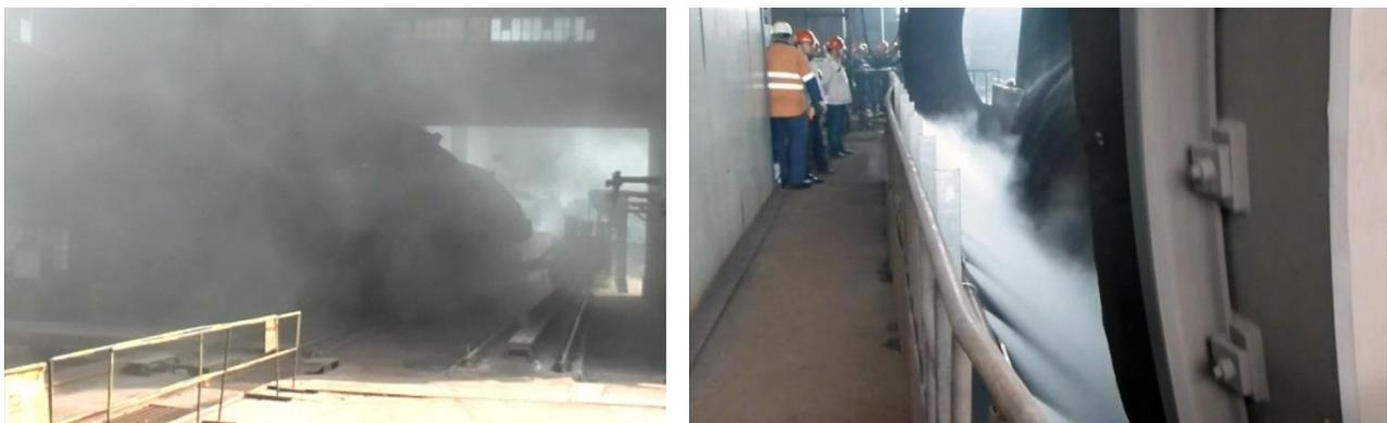
**Figure 6:** Rotary Car Dumper with excessive Dust Emissions (left) and efficient Dust Suppression (right)
