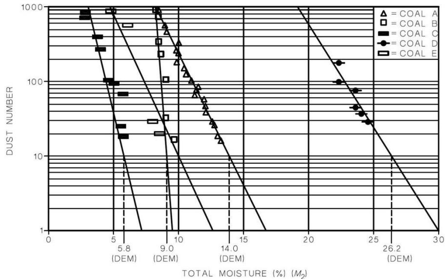
**Figure 3:** Dust/Moisture Curves for Australian Coal, showing DEM = 5.8 to 26.2% wb (AS4156.6, 2000)
