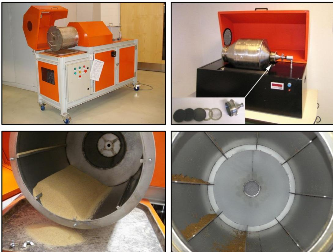
**Figure 2:** Rotating Drum Dustiness Testers: AS4156.6 (2000) (left); EN15051-2 (2013) (right)
