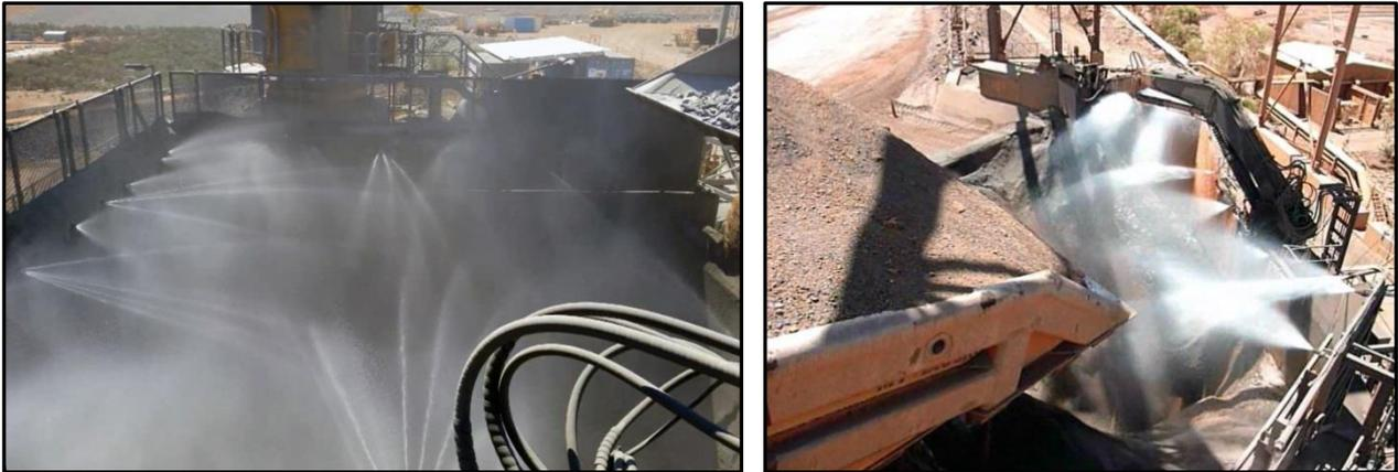
**Figure 1:** Examples of ROM Bin Water Spraying Systems
