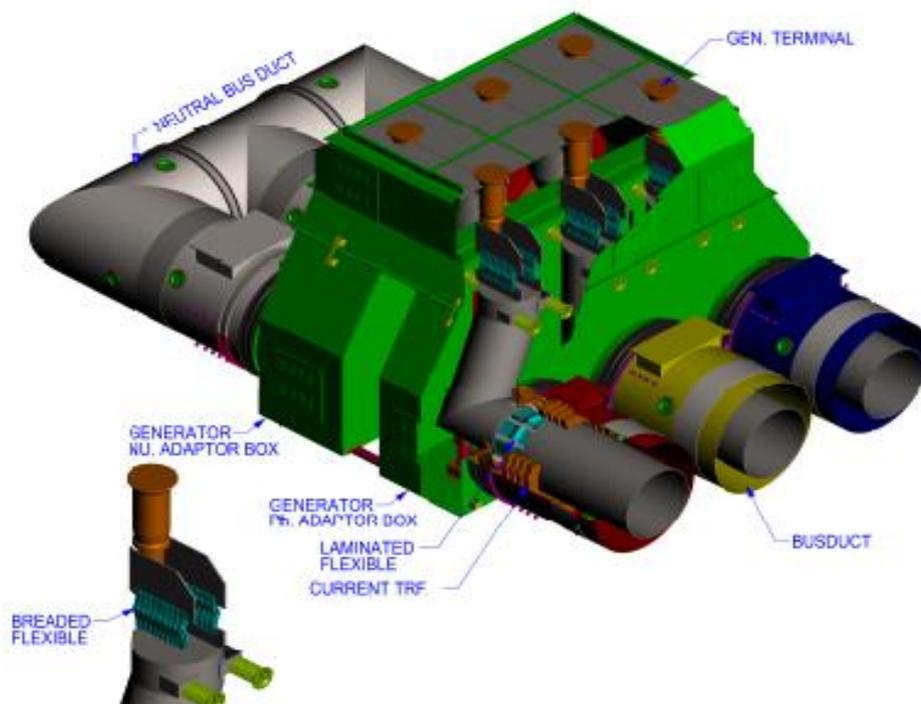
5-(b) Generator Connection with Terminal adaptor Box for Line side/ Neutral side
