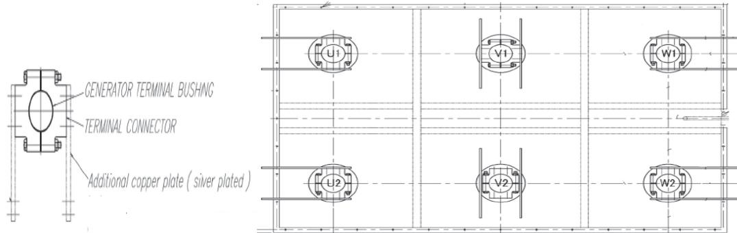
(6) Termination arrangement with copper plates as connection surface
