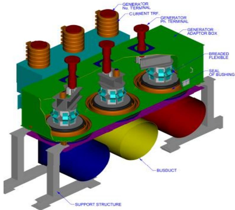
5- (a) Generator Connection with adaptor Box for Line side only ( Neutrals are shorted at Generator terminals itself)
