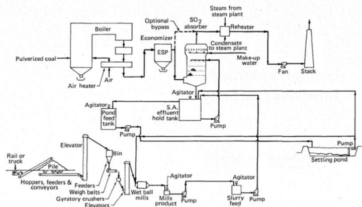
**Figure1:** Limestone slurry process flow diagram
