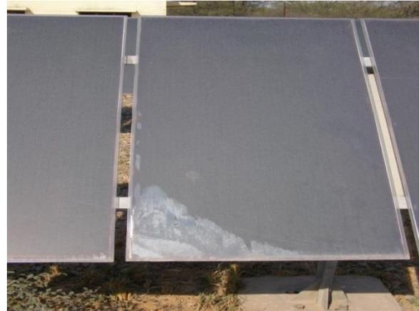
*Figure 3: PV Module indicating Cracks*
