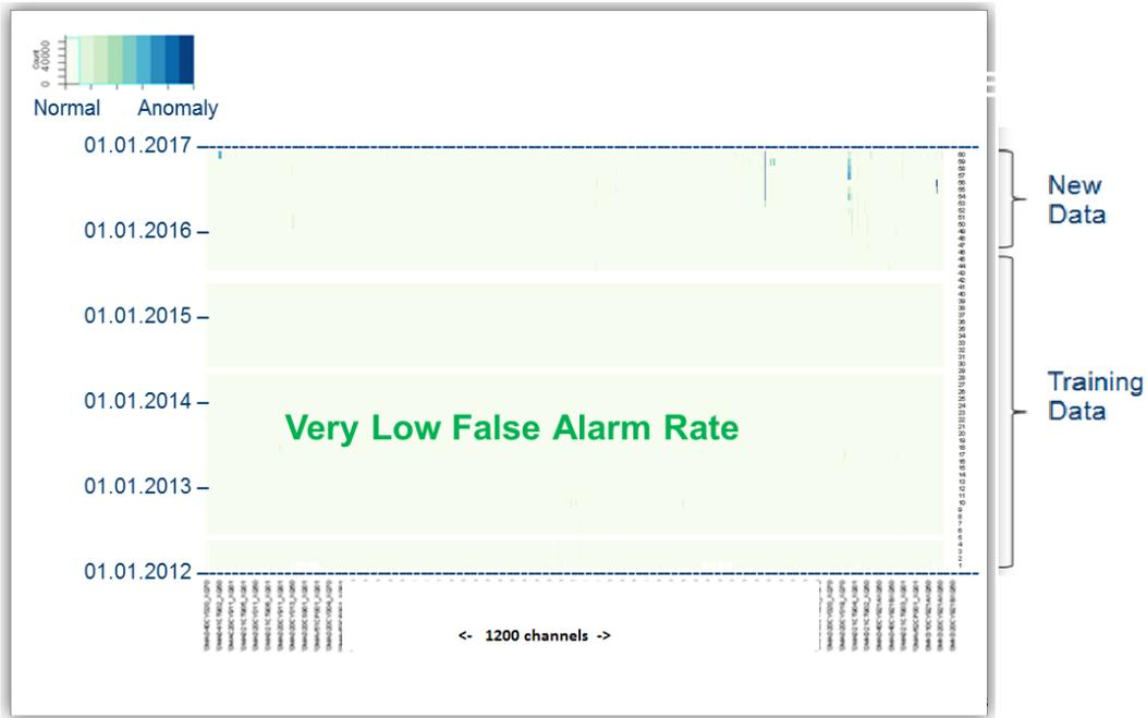
Figure 3: Heat Map for 800 MW unit
