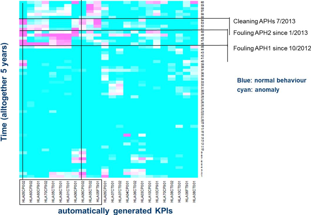
Figure 2: Heat Map for 350 MW unit
