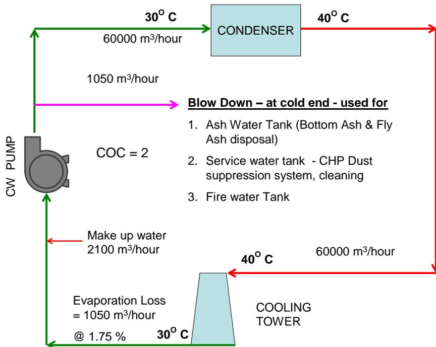
**Figure 1. Present system of Blow down (cold water side)**
