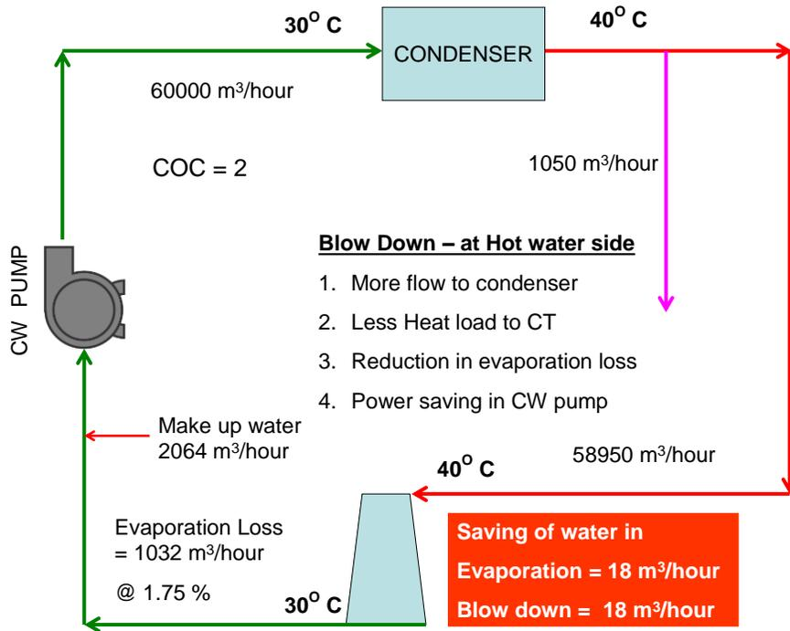
**Figure 2. Proposed system of Blow down (Hot water side)**
