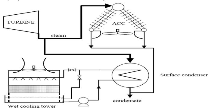
Figure 5.1 : Parallel condensing system (Dry/wet cooling system).
