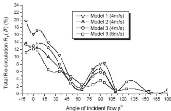
Figure 8.2 : Total re-circulation  $R_T(\beta)$  varies with the angles of incident flow,  $\beta$ .
