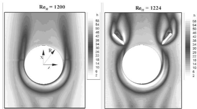
Figure 7.2 : Direct comparison of local heat transfer distributions for a circular cylinder with and without winglets.
