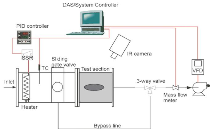
Figure 7.1 : Schematic of flow loop.
