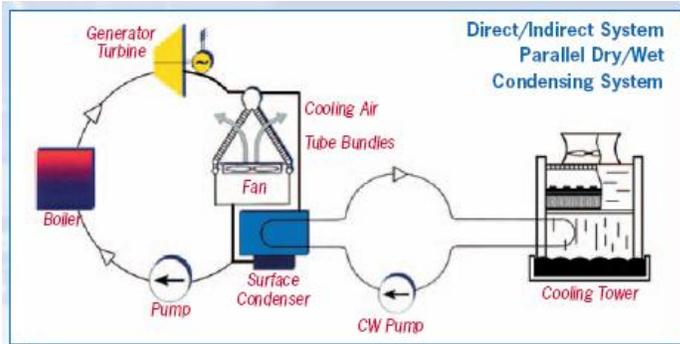
Figure 3.2 : Parallel condensing system
