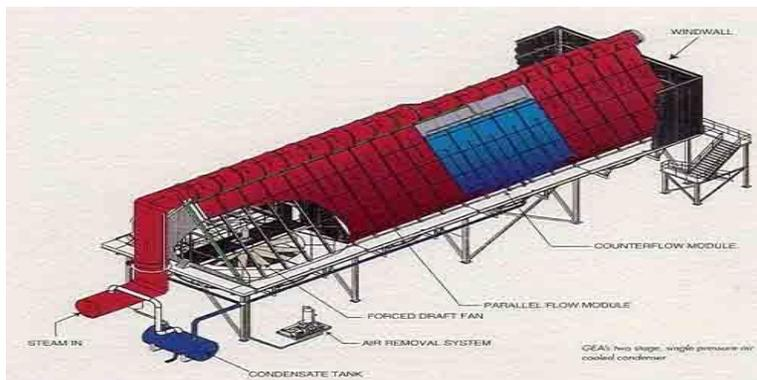
Figure 6.1 : The GEA air-cooled condenser
