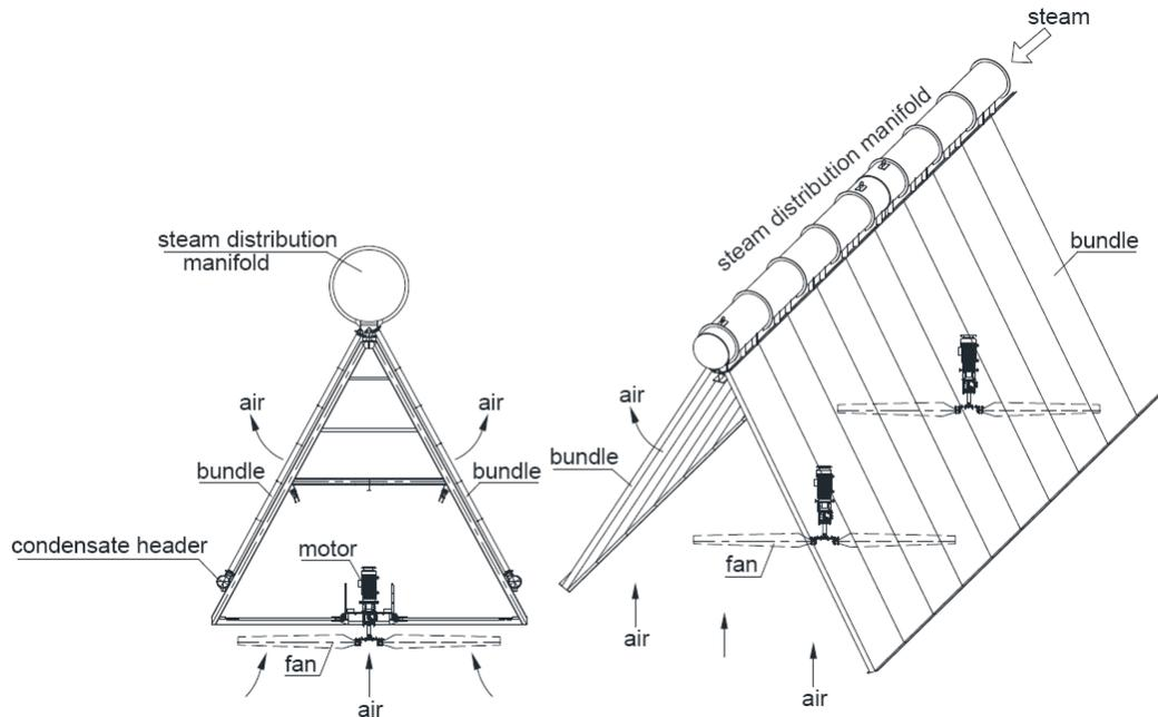
STRUCTURE OF AIR-COOLED CONDENSER OF NTPC NORTH KARANPURA
