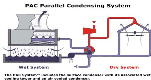
Figure 1.1: parallel condensing system
