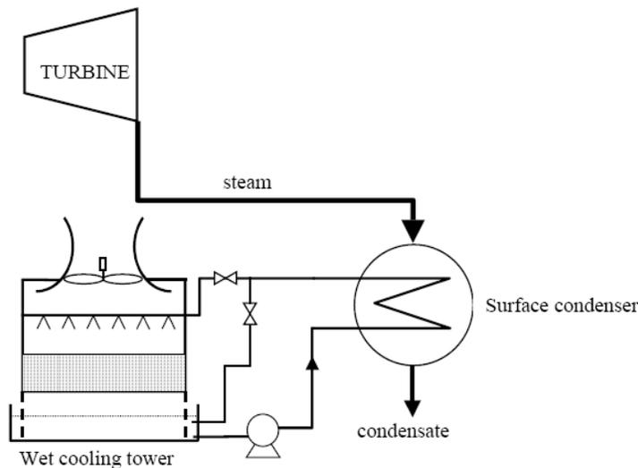
Figure 2.1 : Indirect cooling system with a wet cooling tower and surface condenser.
