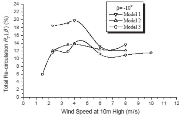
Figure 8.3 : Total re-circulation  $R_T(\beta)$  ( $\beta = -10^\circ$ ) varies with the wind speed for the three models
