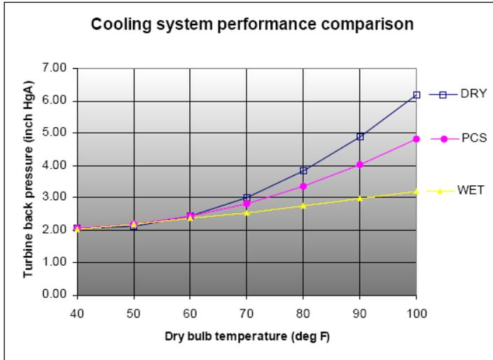
Figure 5.2 : Dry, PCS and wet cooling systems – comparison of the performance.
