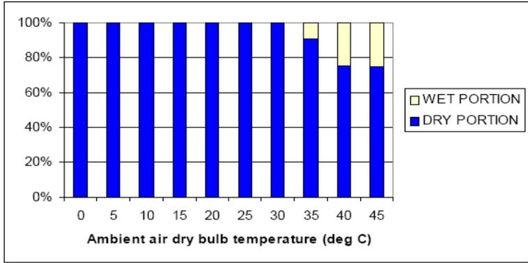
Figure 5.3 : Wet and dry portion of the thermal duty as function of ambient dry bulb temp.
