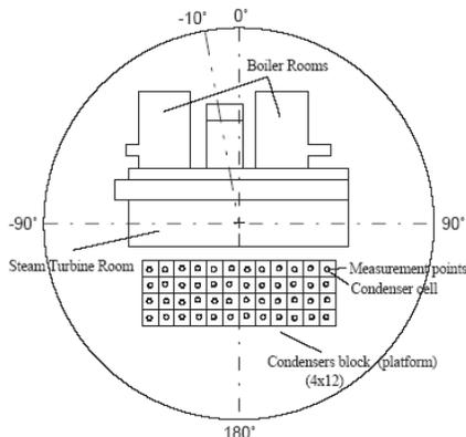
Fig. 8.1 : Schematic configurations of the proposed power plant together with the definition of the angles of incident flow, beta.
