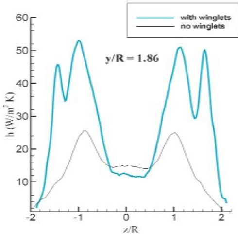
Figure 7.3 : Span-wise variation in local wake-region heat transfer coefficient, with and without winglets.
