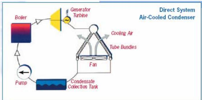
Figure 3.1 : Direct system air-cooled condenser
