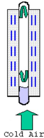
Figure 4.4 : Steam in contact with condensate in SRC tube
