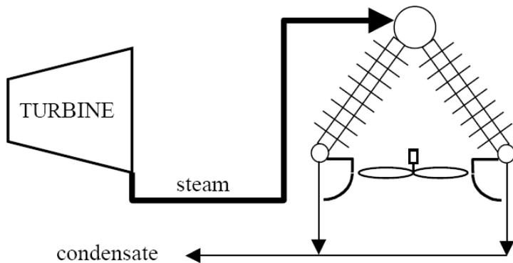
Figure 2.2 : Dry cooling system connected to steam turbine (direct system).
