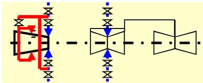
Fig: 8 Provision of Overload valve
