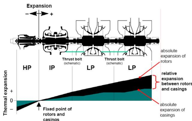
Fig:6 Expansion diagram with self-compensating nature
