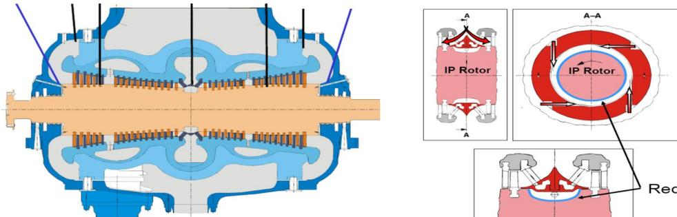
Fig: 5 Thermal shield for IP turbine (Courtesy Siemens / BHEL)
