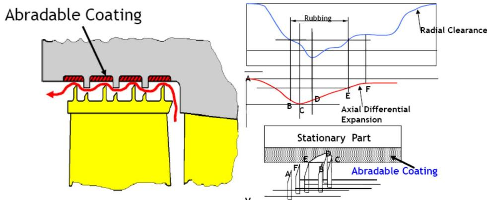
Fig: 7 Abradable seals (courtesy:- Toshiba)
