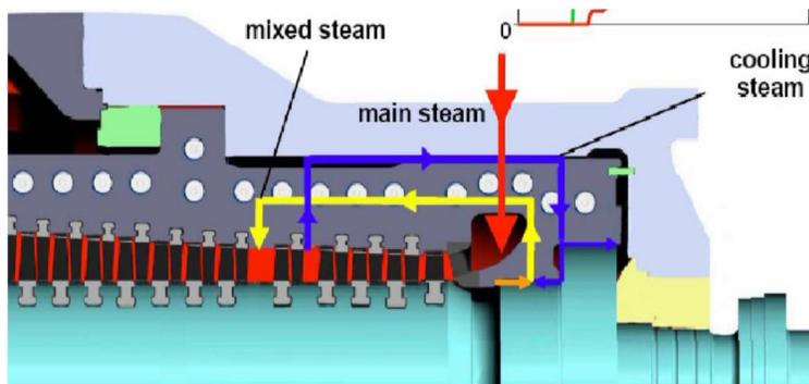
Fig4:- HPT internal cooling arrangement (Courtesy- Siemens/ BHEL ltd.)
