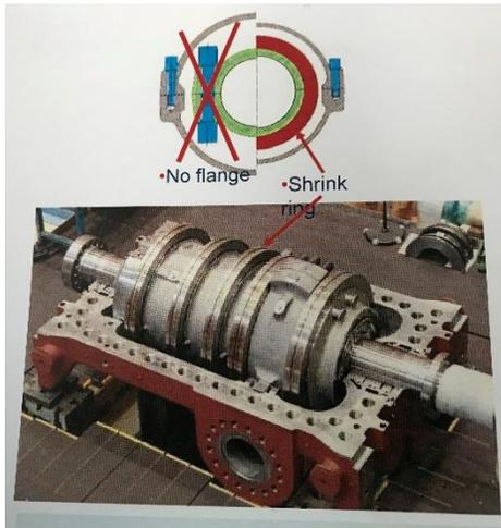
Fig: 2 Shrink ring HP turbine inner casing (Courtesy GE)
