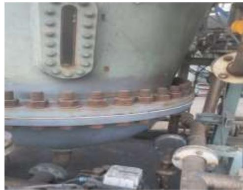
fig 3: Before & after modification. Flange was provided at ARU to hold the matrix.
