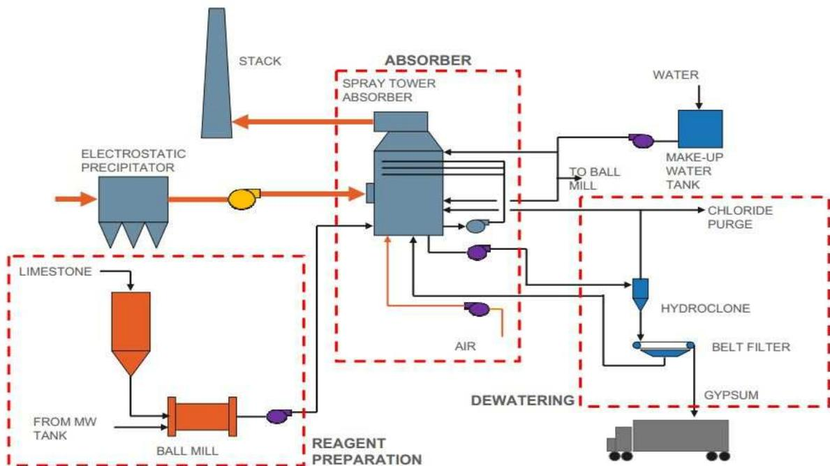
Fig (4): Typical Flow diagram of wet FGD system
