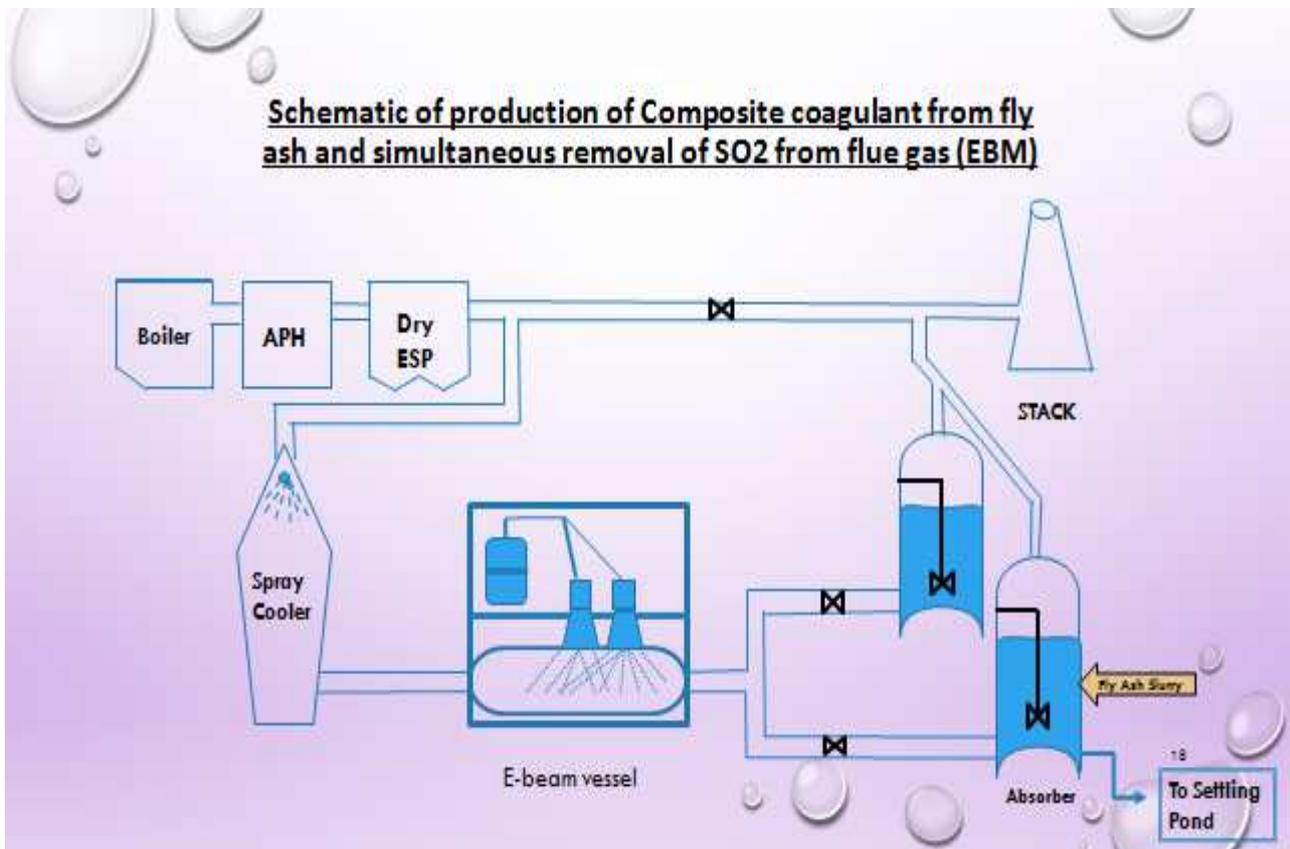
Fig (5) Typical Flow Diagram of removal of SO<sub>x</sub>/No<sub>x</sub> from flue gas by E-Beam method
