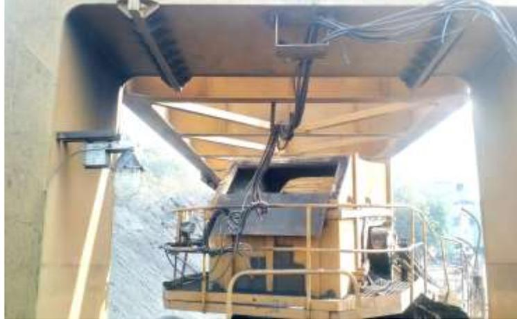
Fig.2. Profibus cable routed outside the inner slew ring
