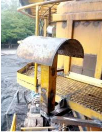
Fig.6:- Hinge support for Cable movement
