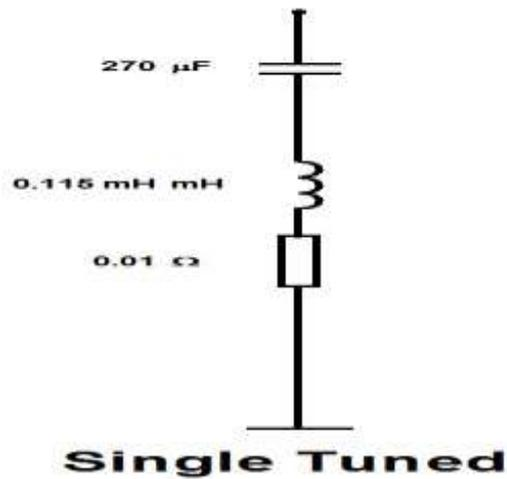
**Figure 3: 18<sup>th</sup> Single-Tuned Filter at 1100V**
