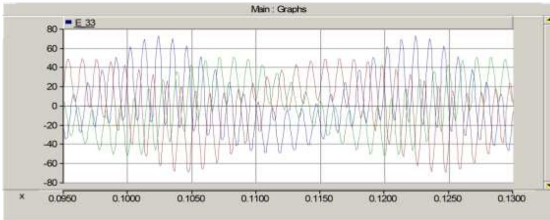
Figure 5 : Voltage Spectrum – with 1100V Filter
