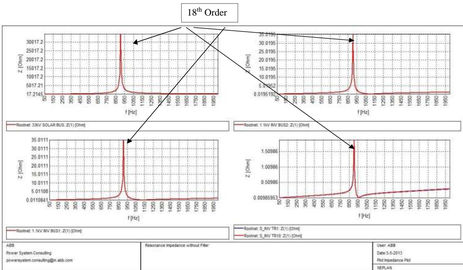
**Figure 2: Frequency Scan – Normal System Configuration without Filter**
