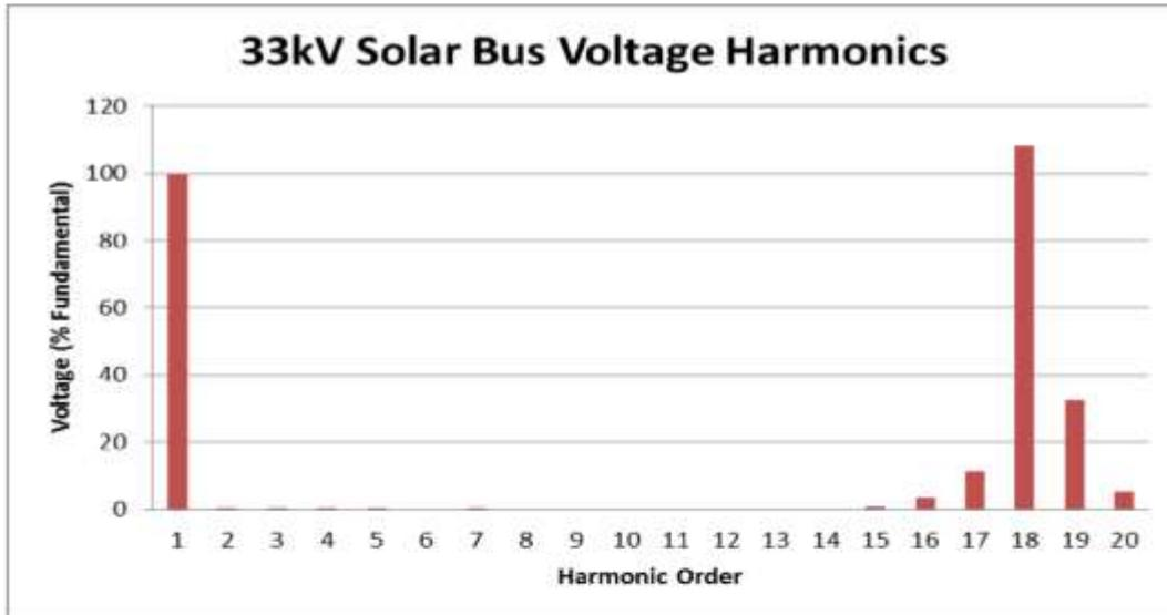
Figure 4-1 Voltage Spectrum – Without Filter
