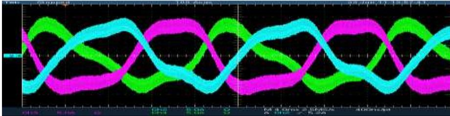
**Fig 1: Distortion due to Harmonic resonance between inverter and grid**
