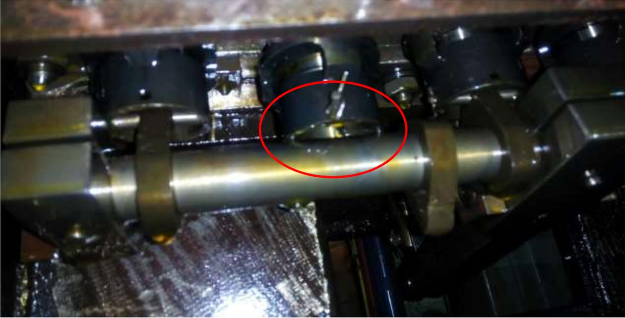
Fig-7: Dislodged split pin and cylindrical pin of IP follow-up piston in EHC
