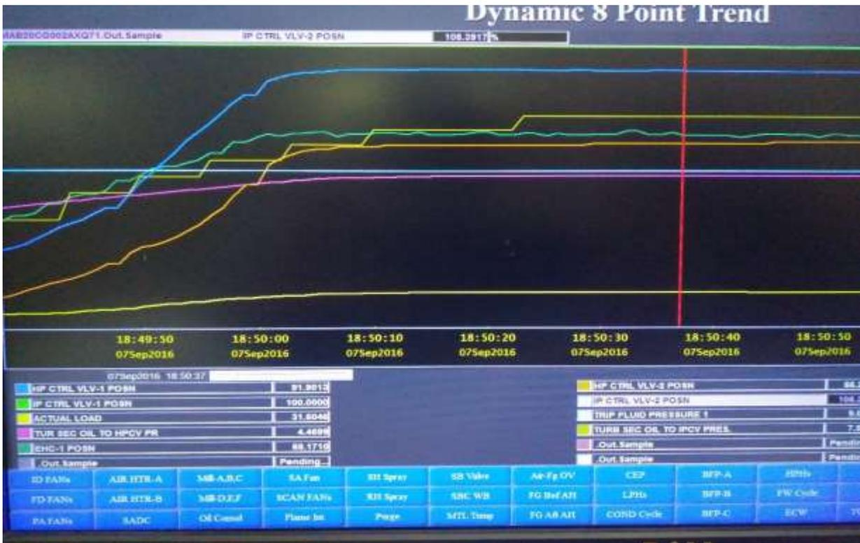
**Fig-4: Pressure and Load Trends before the incidence**
