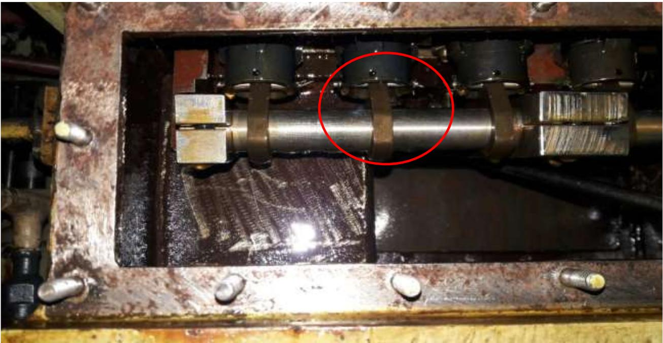
Fig -8: Split pin and cylindrical pin of IP follow-up piston in EHC after replacement
