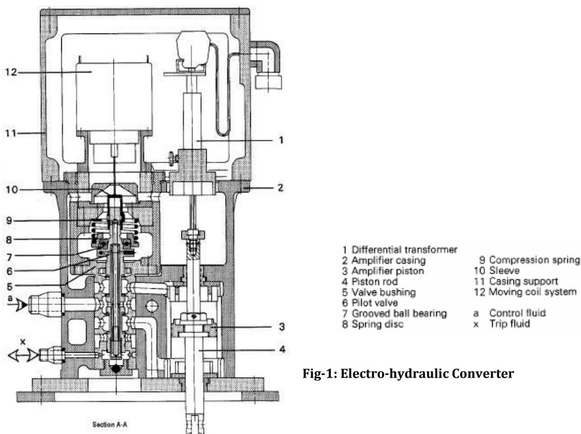
Fig-1: Electro-hydraulic Converter
