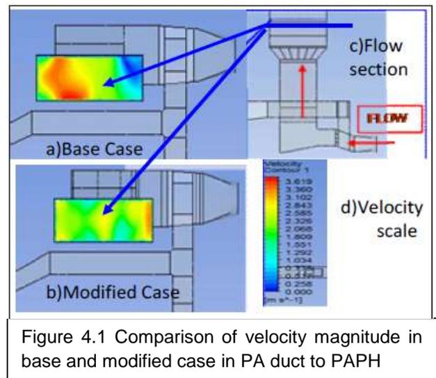
Figure 4.1 Comparison of velocity magnitude in base and modified case in PA duct to PAPH
