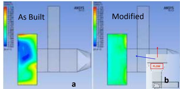
Fig 4.2 Comparison of velocity at SA duct from FD fan to SAPH inlet
