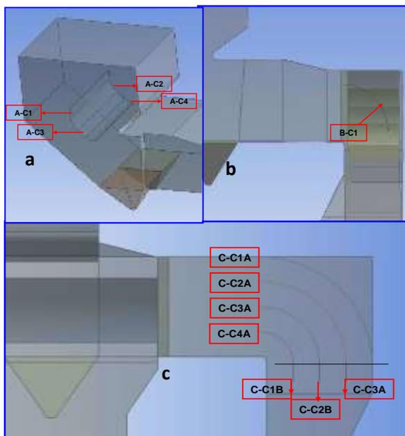
Figure 3.1 Optimized modification simulated in Flue gas duct from Economizer outlet to inlet of PAPH and SAPH
