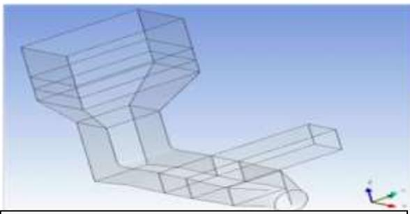
Figure-2.2: Isometric view of 3D model of air duct from FD fan outlet to SAPH inlet
