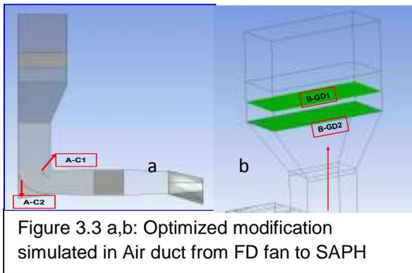
Figure 3.3 a,b: Optimized modification simulated in Air duct from FD fan to SAPH
