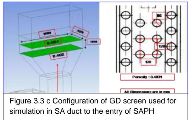
Figure 3.3 c Configuration of GD screen used for simulation in SA duct to the entry of SAPH
