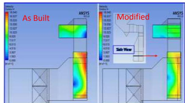
Fig 4.3b Comparison of velocity at FG duct inlet to SAPH and PAPH for base and modified case. The section seen is horizontal plane passing above the SAPH/PAPH FG entry
