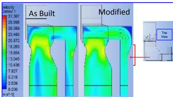
Fig 4.3a Comparison of velocity at FG duct inlet to SAPH and PAPH for base and modified case. The section seen is vertical plane passing through mid-section of PAPH/SPAPH
