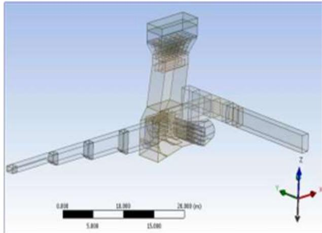
Figure-2.1: Isometric view of 3D model of air duct from PA Fan outlet to PAPH inlet
