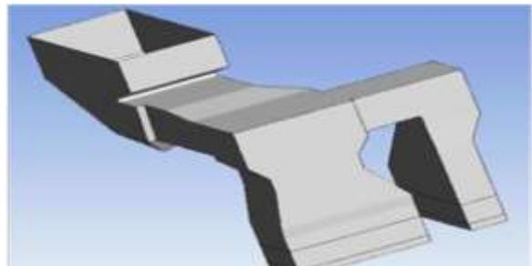
Figure-2.3: Isometric view of FG duct section from Economizer outlet to APHs inlet
