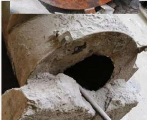
Damaged Silencers due to corrosion/erosion
