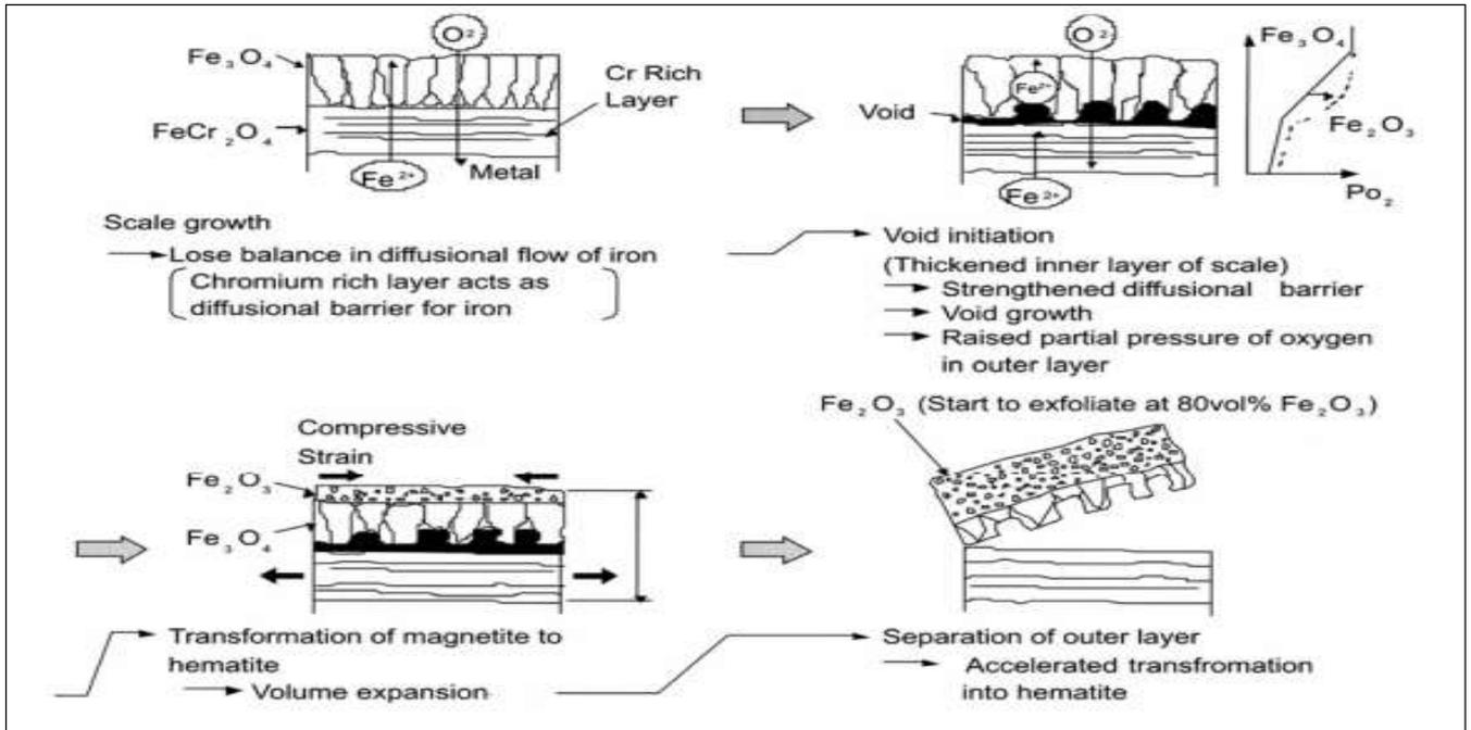
**Fig : Schematic Representation of the Usual Sequence of Events in the Exfoliation of Scale**
