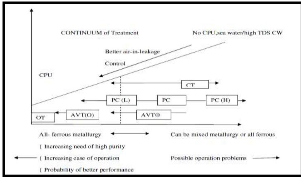
**Fig- General guidelines for boiler feed water chemical treatment system**
