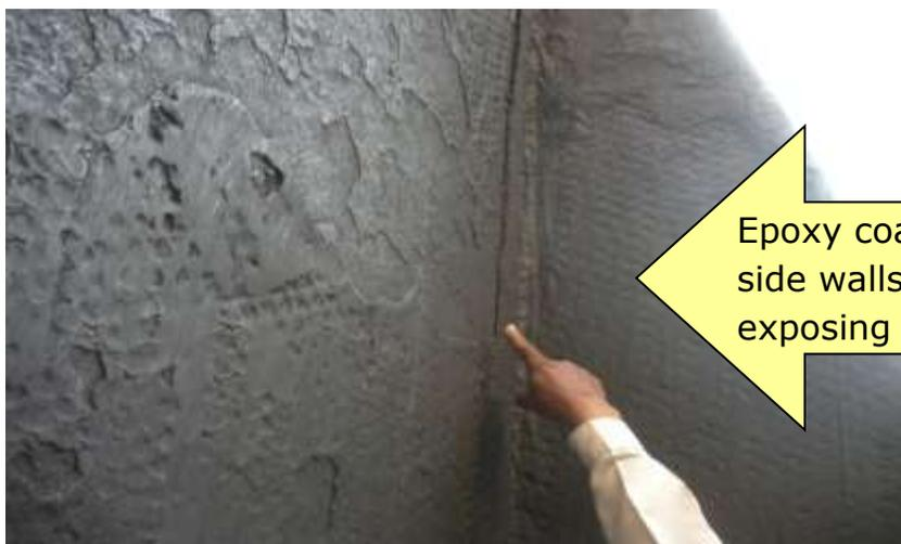
Epoxy coating peeled off from side walls of wagon body exposing parent material
