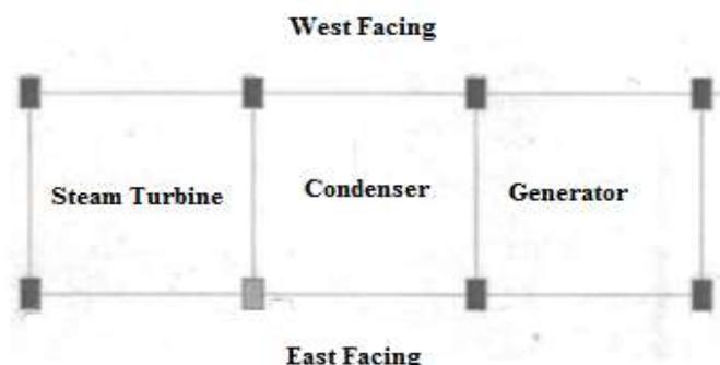
Fig. 1: Typical plan of RC Columns located in power house near sea shore in India
