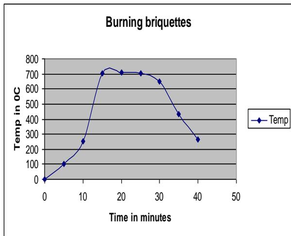
**Figure 7:** burning residence time Vs temperature
