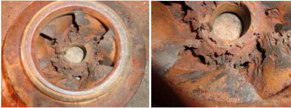
Fig. 5 & 6: Severely Corroded and Cavitation affected Impeller Blades of Pumps
