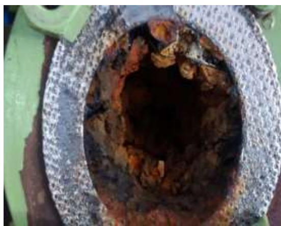
Fig. 14: Tubercles in cooler sample pipe
