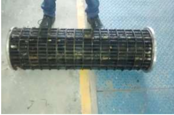
Fig. 11: Compressor Cooler – Fouling & deposition
