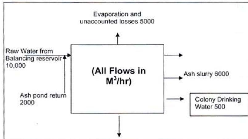
Figure 2: Water balance for a super thermal power plant
