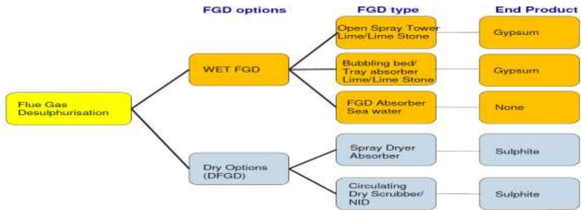
Fig.2 Types of FGD systems.
