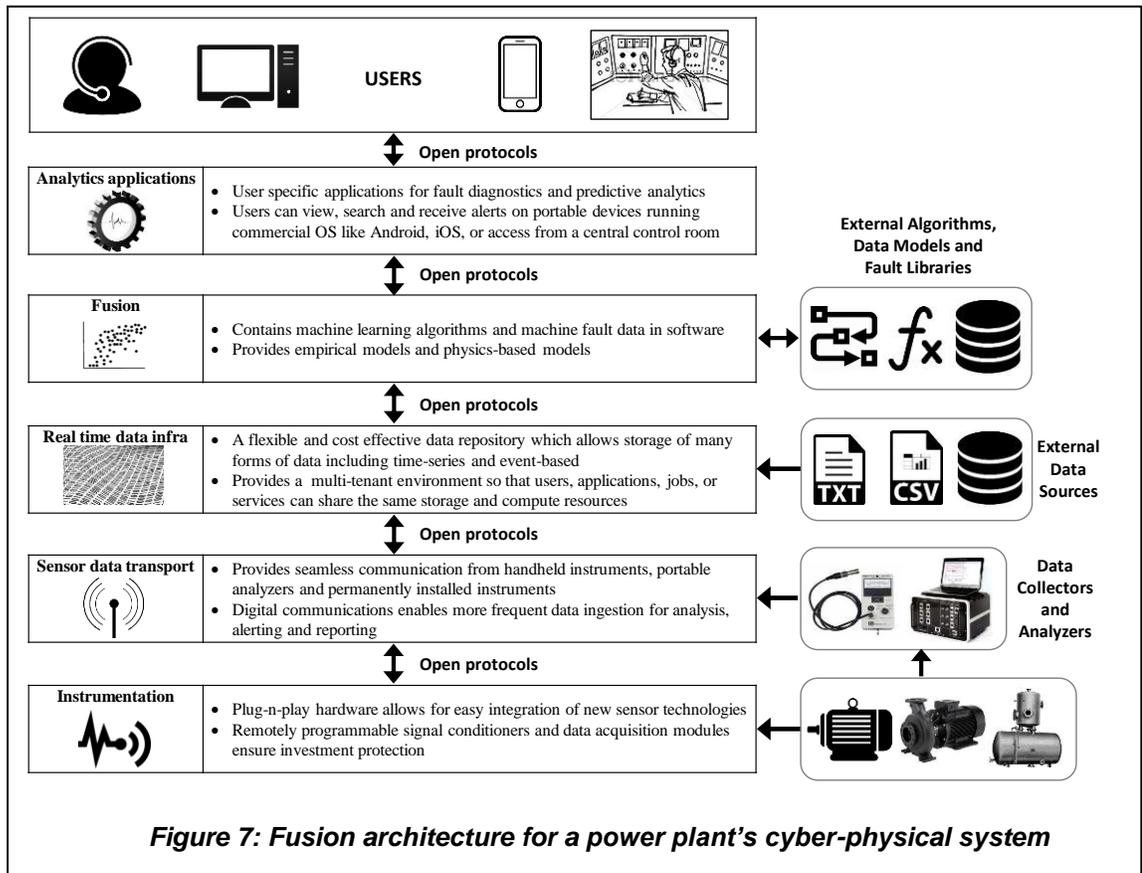
From an implementation perspective, we can rapidly create and prototype a multivariate model to predict failures within a predefined window before equipment/machinery encounters anomalous behavior or actually fails. We recommend that end users adopt the data science process for predictive maintenance: prepare the dataset, visually explore it, partition the data for training and testing, validate the models using previously unseen data, and finally deploy the model.
