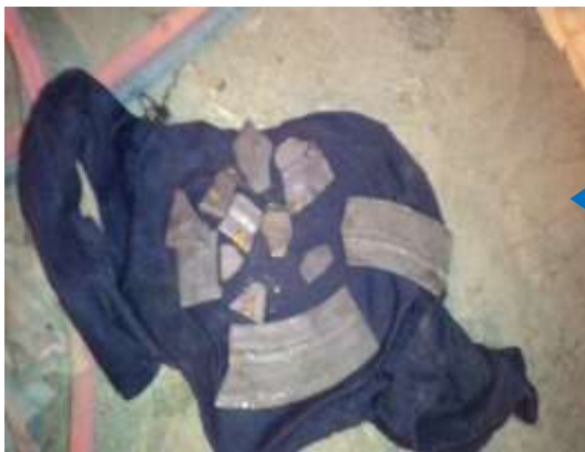
MS valve stellite liner pieces in
