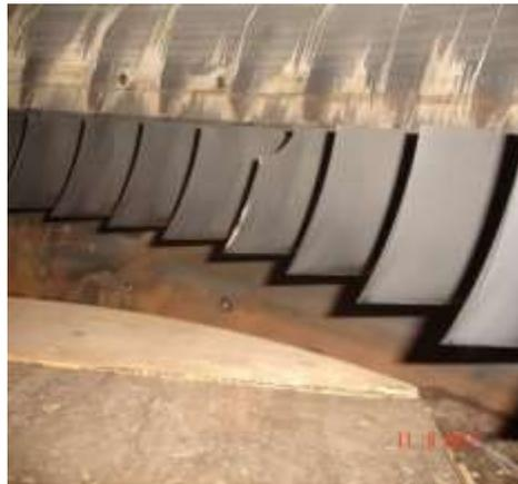
After inspection it was observed that FOD event occurred in R1 blades-19 and 24 chipping off portion of the blade tip at the leading edge. Thus, catastrophic failure was saved with the help of BHM.
