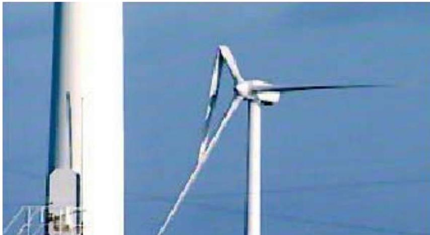
Fig.7 – An example of blade damage at 30% from root
