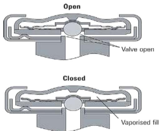
**Fig. 5 Operation of balanced pressure steam trap capsule**
