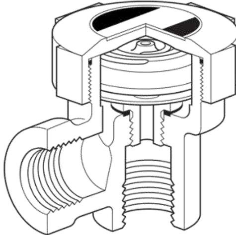
**Fig. 4 Balanced Pressure Steam trap**
