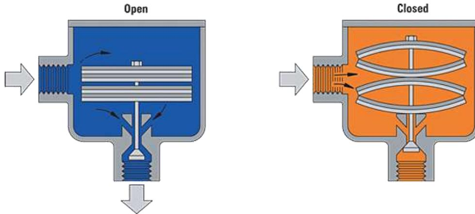
**Fig. 6 Operation of a bimetallic steam trap**
