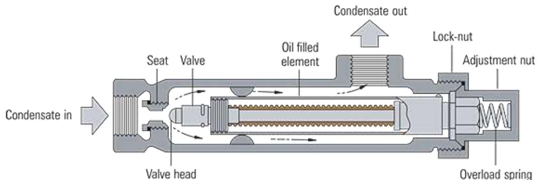
**Fig. 3 Liquid Expansion Steam trap**
