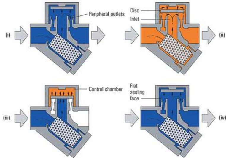
**Fig. 7 Operation of Thermodynamic steam trap**
