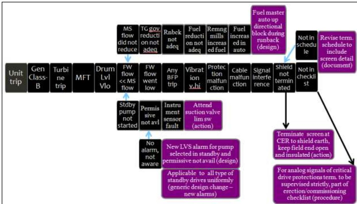
**Figure-5 : RCA software entry demonstration for C&I trip case study (completed snapshot)**
