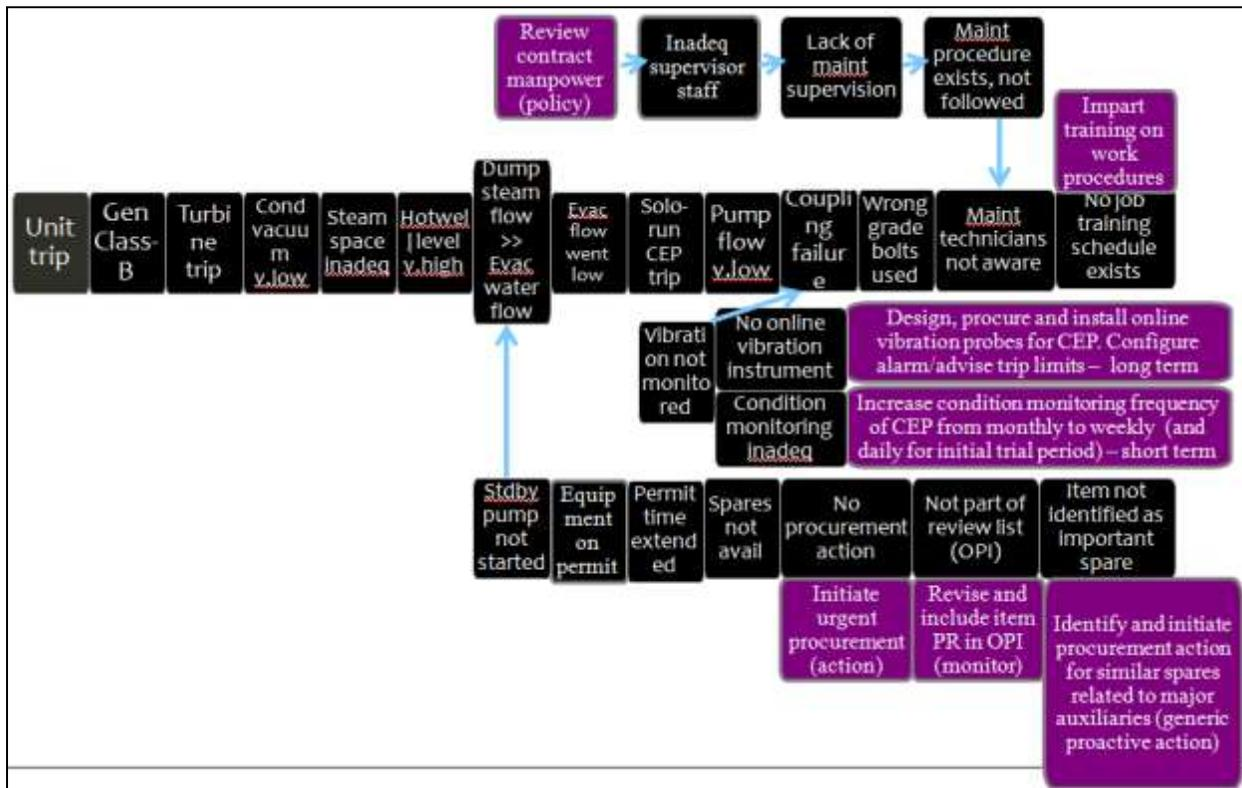
Figure-6 : RCA software entry demonstration for mechanical trip case study (completed snapshot)
