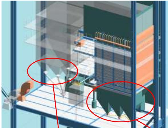
Below *Picture 3* visualize the retrofit of the SCR in the 2<sup>nd</sup> boiler path. On the left side of the picture the original situation is shown. On the right side the layout after integrating the SCR reactor and ammonia injection system is indicated.
