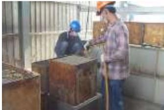
In the next step the catalyst was regenerated in a 2 step washing process including re-coating of the catalyst. Due to a dust removal step in the washing water, the water management could be optimized. The waste water was treated by the existing plant in the Power Station and had a similar characteristic as the air-pre heater washing water.
