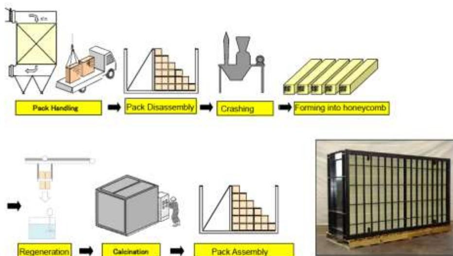
**Figure 3-4 Regeneration steps of Honeycomb type Catalyst**
