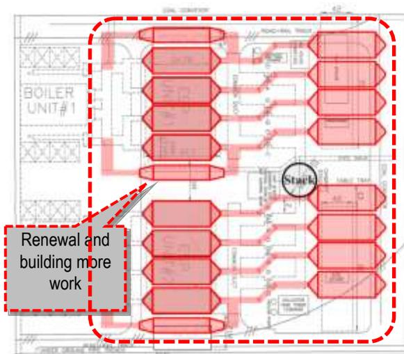
**Figure 2-2 Rihand TPS site layout (Conventional type ESP plan)**
