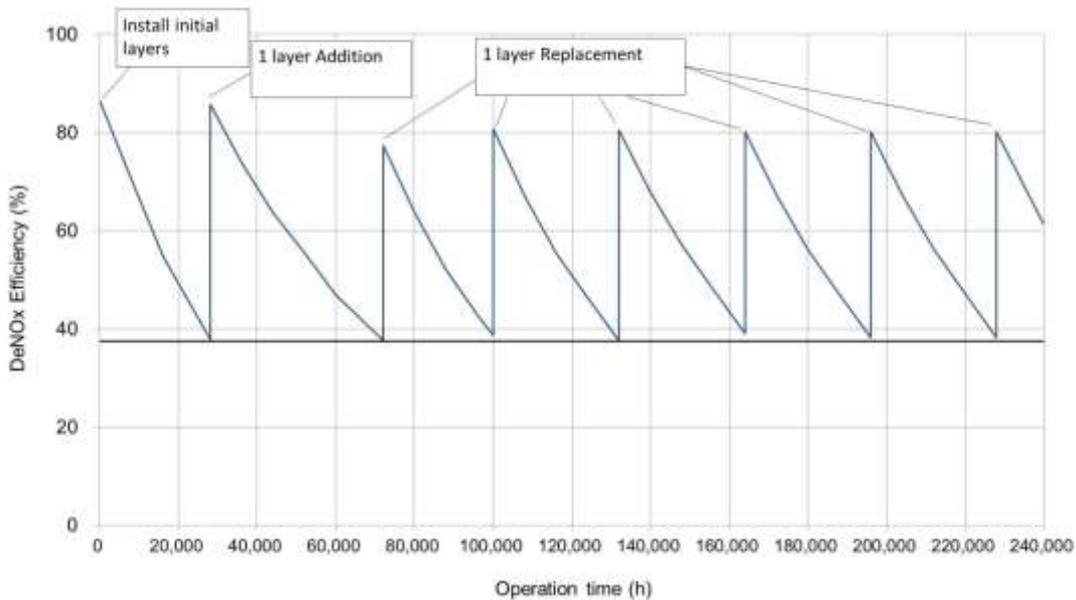
**Figure 3-2 Typical Catalyst Management Plan**
