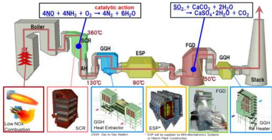
Fig. 1-1: Air Quality Control System components
