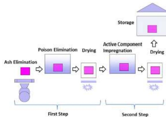
**Figure 3-3 Regeneration steps of plate type Catalyst**
