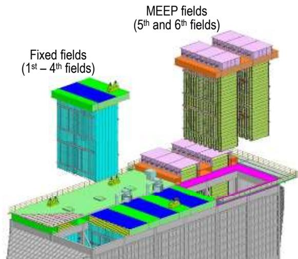
**Figure 2-3 Retrofitting in existing ESP using the MEEP**
