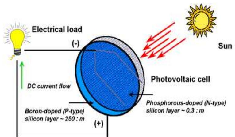
Figure 1. Diagram of a Photovoltaic Cell
