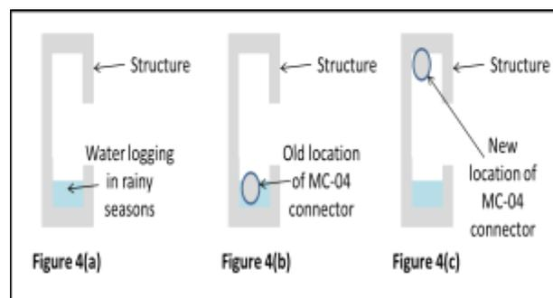
Figure 2. Location shifting of MC-04 connector
