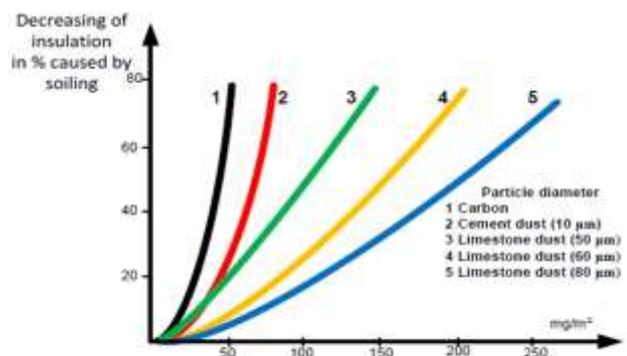
Fig 5: Effect of different particle pollutants to the energy loss
