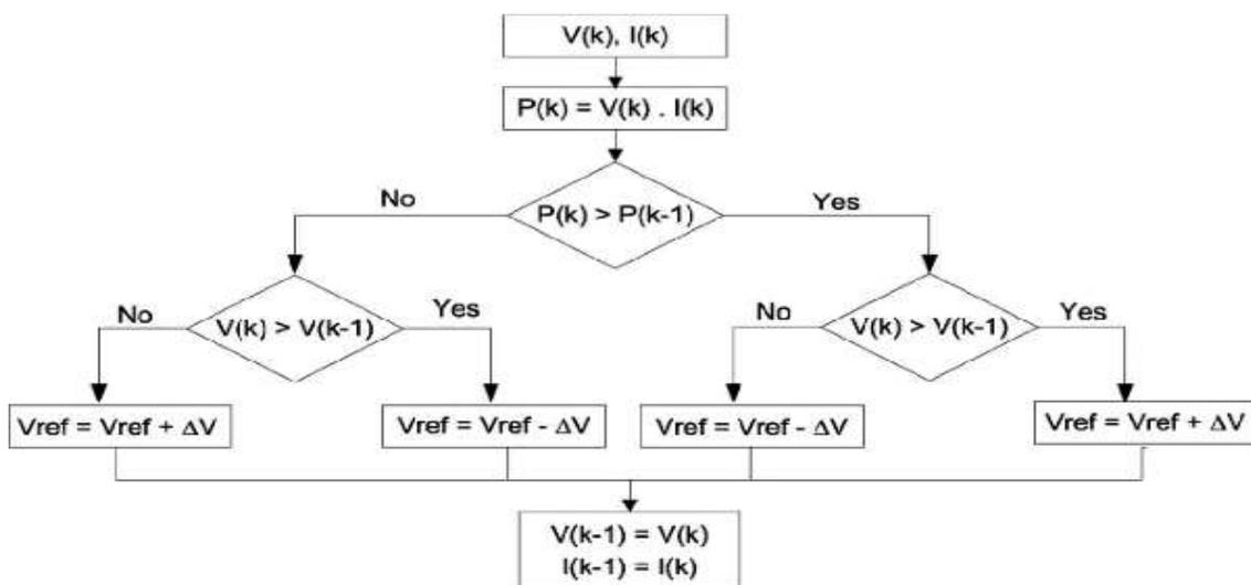
Figure5: Flowchart of Perturb and Observe
