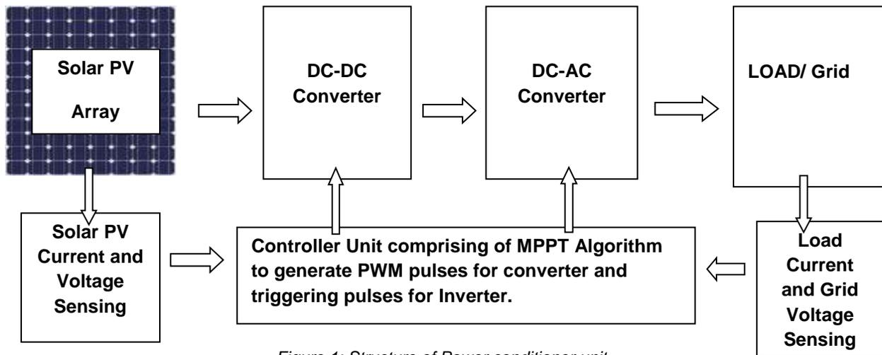
Figure 1: Structure of Power conditioner unit
