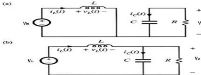
Figure6: (a) Switch in ON state (b)Switch in off state
