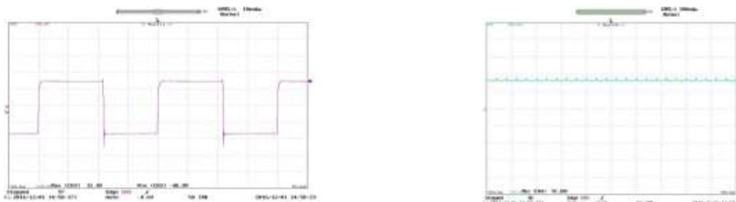
Figure 10: hardware result waveform for a) voltage across inductor b) current through inductor
