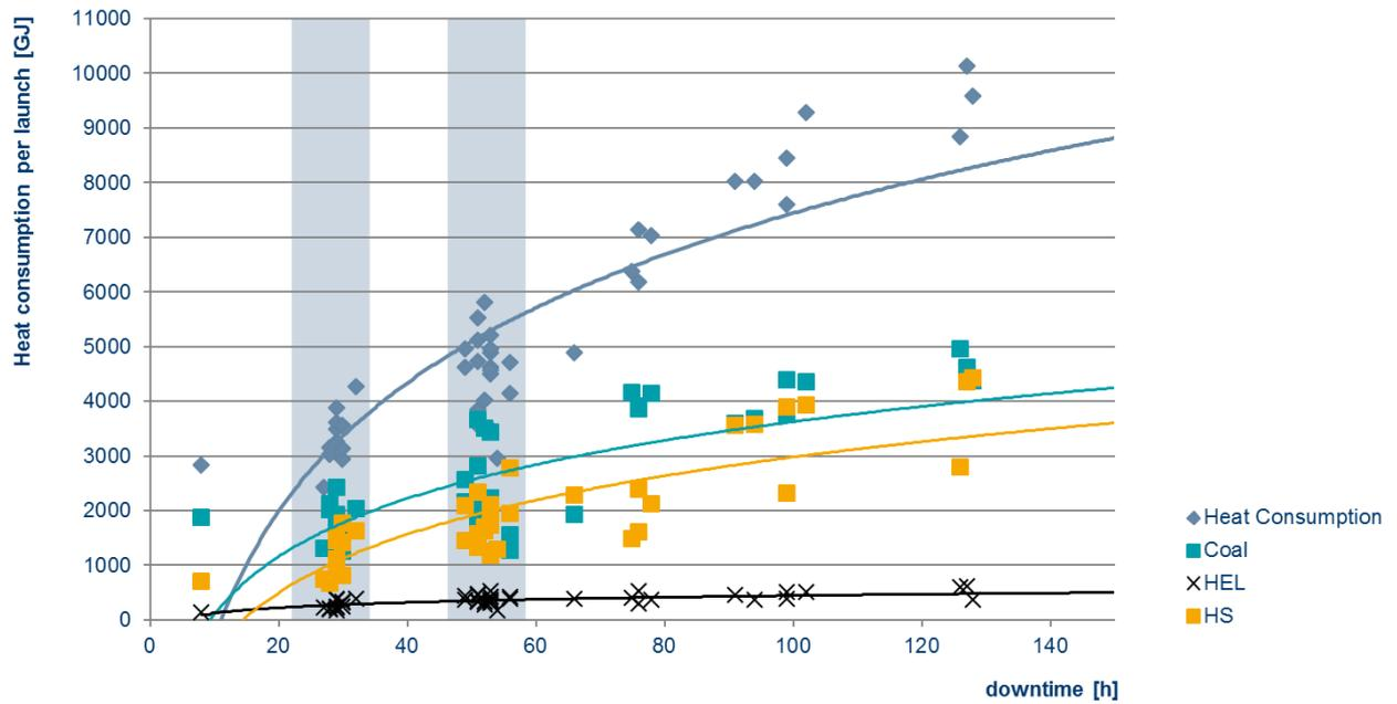
Fig. 1: Fuel and heat consumption for different start-up procedures as a function of the downtime
